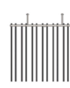
Safety grille bars
