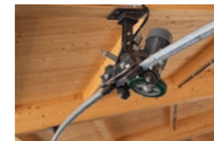
Drive system for round ring horse walker
