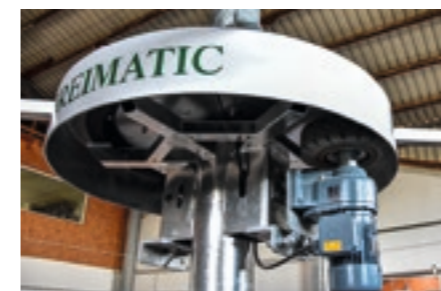
Drive system for tower horse walker
